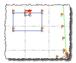
If the coordinates for an as-staked point and its corresponding design point are not within the tolerances you specified in the **Project Settings** dialog, the as-staked point includes an out-of-tolerance flag. In this project, a red flag is displayed for each as-staked point whose horizontal tolerance exceeds 0.20 ft.
