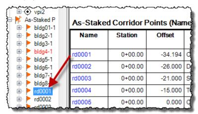
Red text for station deltas (1 below) and offset deltas (2) indicates the as-staked point is out of horizontal tolerance and has been flagged in the project.
