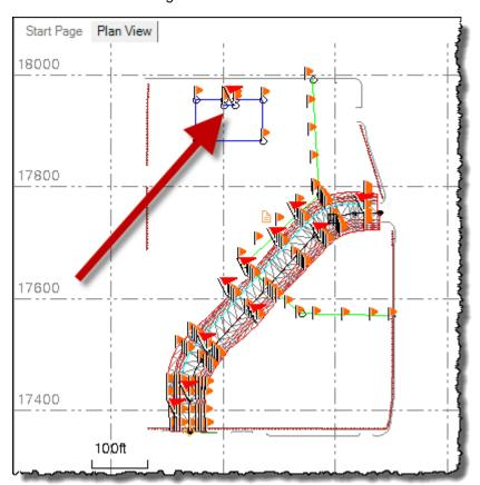
Zoom in farther until the as-staked point (1 below) and its corresponding design point (2) are clearly visible.
