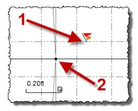
You can see that the as-staked point is approximately 0.20 ft out of horizontal tolerance with the centerline at station 5+36.89.
