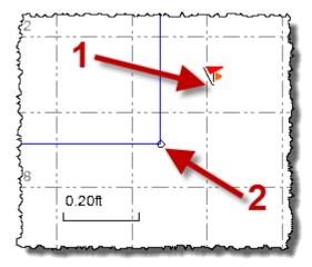
You can see that the as-staked point is approximately 0.20 ft out of horizontal tolerance with the design point.
