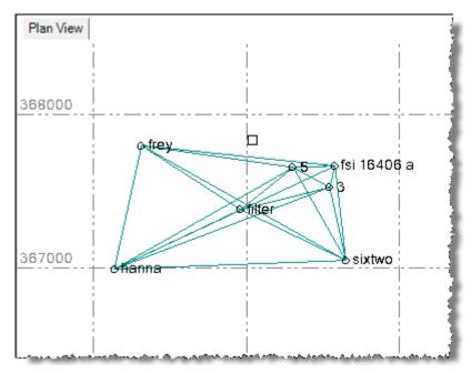
The GNSS static data is imported into your project and displayed on the **Plan View**.
